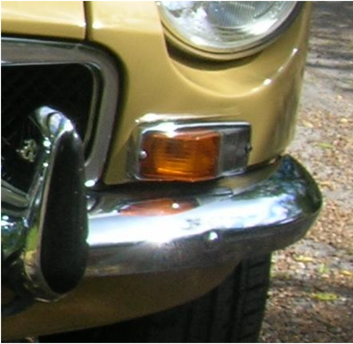
On this chrome bumper grille the V8 badge is too high and too far to the nearside of the grille. Note also the restorer has got the sidelight-indicator light unit the wrong way round too! The side light should be on the outside marking the edge of the front of the car and the indicator inside.
