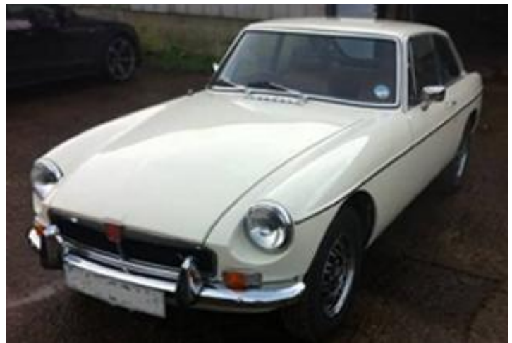
On this chrome bumper grille the V8 badge is too high and too far to the nearside of the grille. Note also the restorer has got the sidelight-indicator light unit the wrong way round too! The side light should be on the outside marking the edge of the front of the car and the indicator inside.
